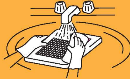
2. Wash and clean louver.
