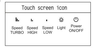
\*\*Speed TURBO: under Speed TURBO, the motor will operate in ultimate speed and can increase suction instantly.
