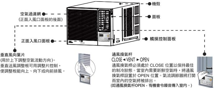
空氣過濾網 (正面風口面板的後面)
