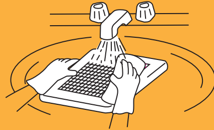
2. Wash and clean louver.
