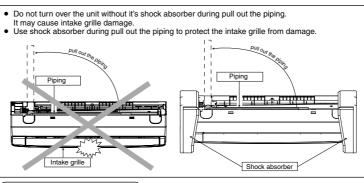
. FOR THE RIGHT REAR PIPING Right Rear piping Pull out the Indoor piping ape it with piping in a position as entioned in Fig. below. Install the Indoor Unit Secure the Indoor Unit If indoor power supply, excess length of power supply must arrange accordingly, please refer "Power supply cord arrangement" before secure the indoor unit. How to keep the cove n case of the cover is cut, Step-4 Insert the connection cable keep the cover at the rear of chassis as shown in the illustration for future
