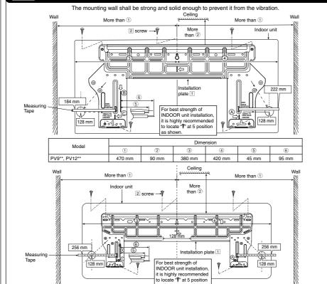
The center of installation plate should be at more than ① at right and left of the wall. The distance from installation plate edge to ceiling should more than From installation plate center to unit's left side is 3.
