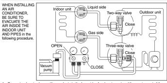
Connect a charging hose with a push pin to the Low side of a charging set and the service port of the 3-way valve.
